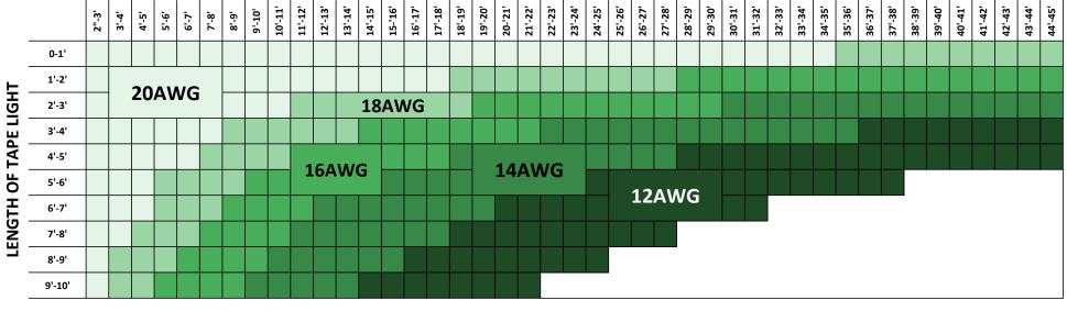
20AWG 18AWG 16AWG 14AWG 12AWG These recommended wire gauges are based on the National Electrical Code (NEC). Please consult with a licensed electrican or recognized authority to verify local code. Select wire gauges are available for purchase.
